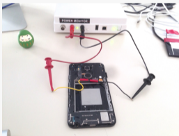
Figure: Example usage of Monsoon Power Monitor 1
